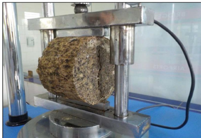
⑫ Broken test specimen showing crack.
