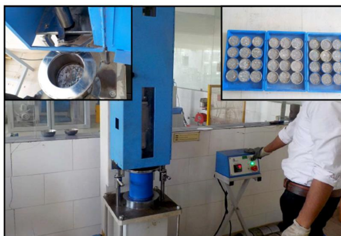
④ Compaction of ITS & Marshall specimen-36 Nos.
