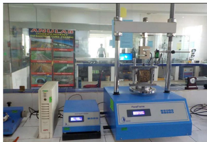
⑩ Automatic ITS testing machine with peak arrest.
