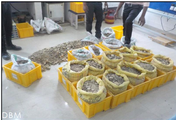
① As received milled RAP from project site.
