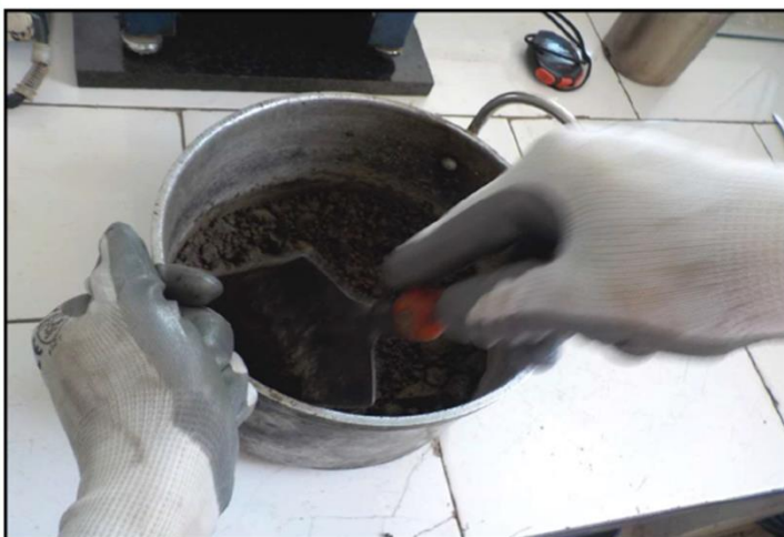
③ Mixing of RAP + aggregate+cement in pan at 22°C
